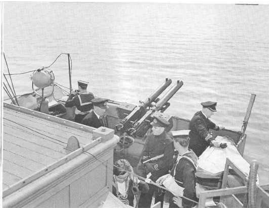
The original corvette bridge, like HMCS Moncton's seen here, during work-ups in May 1942, was ill-suited to the demands of war. The charthouse, in the left foreground, housed the ship's only compass—a magnetic one—and the trace recorder/or the primitive type 123A asdic set, but the captain had to fight his ship from outside and the charthouse itself prevented a full 360 degree view of events. The cramped bridge wings did well to accommodate the twin .50 calibre machine guns seen here.
