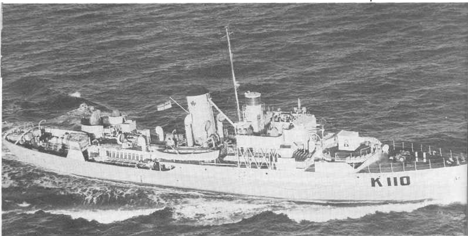
The object of the RCN's desire in 1943: the fully modernized corvette, HMCS Shediac in 1944. Note the hedgehog just forward of the bridge.
