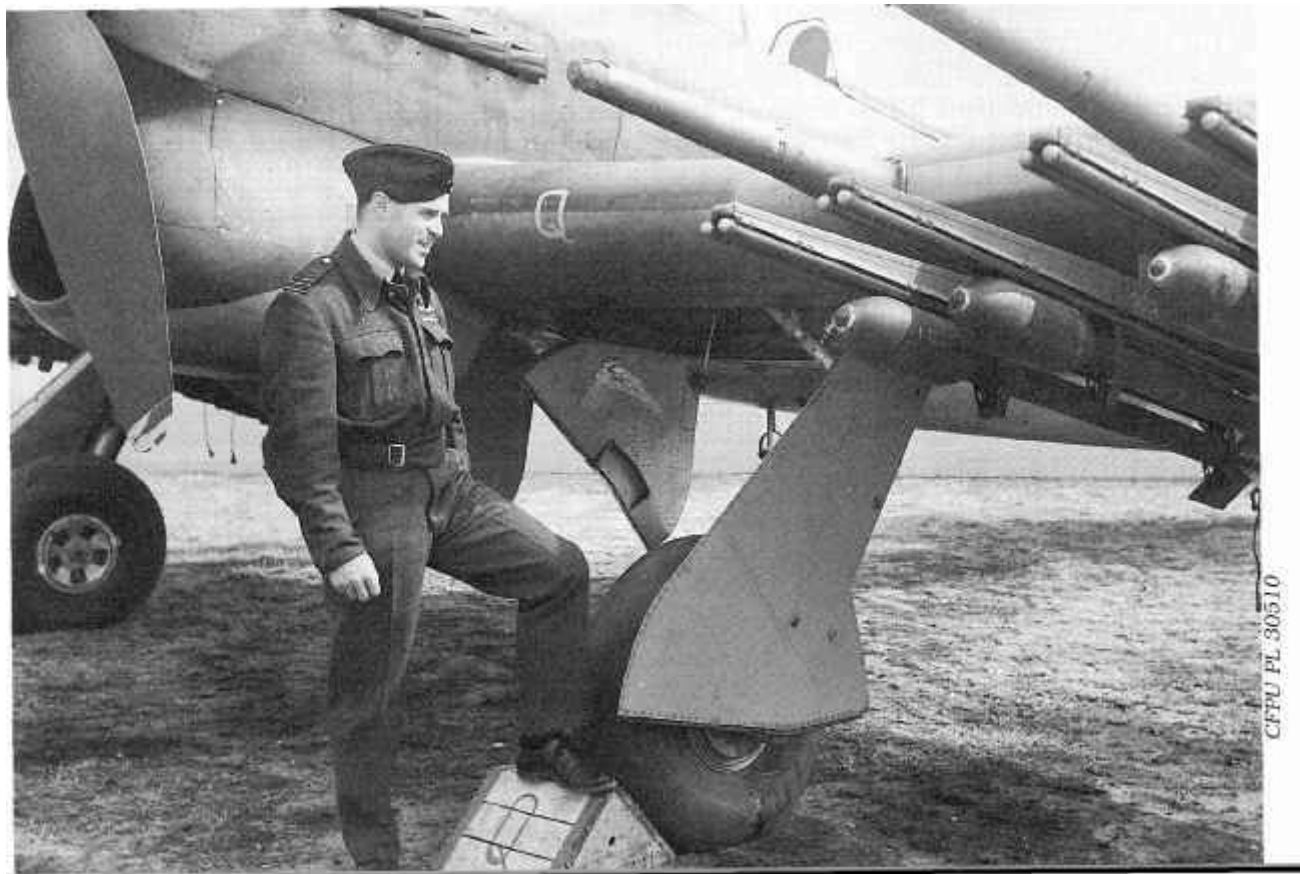
A Canadian Group Captain looks at the offensive punch of the Hawker Typhoon - its Rocket Projectiles.
