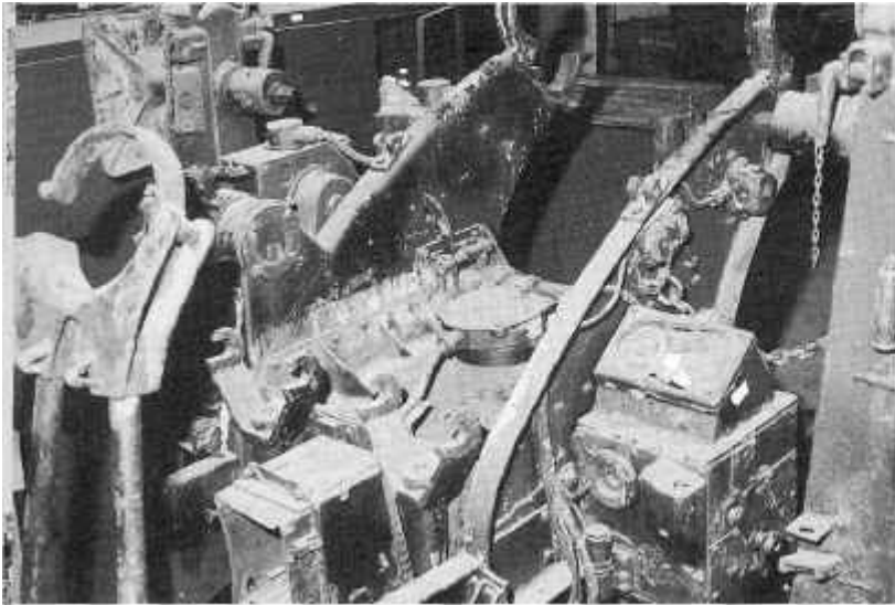
Components of the Canadian War Museum 88 prior to restoration: Above left: The pedestal assembly - virtually every moving component was firmly rusted and seized. Above right: The breech mechanism of the gun. Opposite: The barrel assembly. (Photos courtesy of author)
