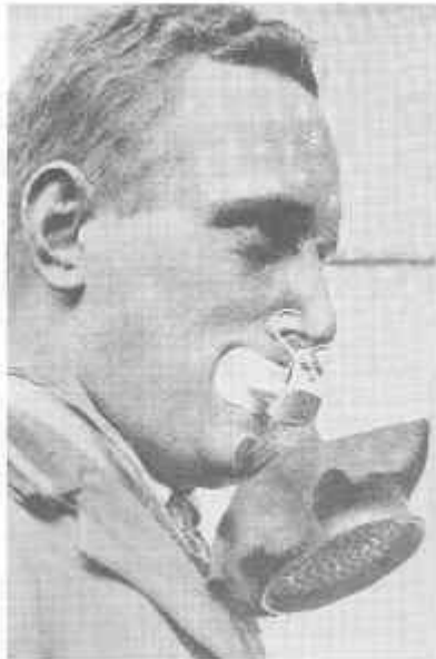
These two photographs shows a German Gas Mask that was captured in mid-1915 by the Canadians. The photograph on the left show it worn with the face mask while the photo in the centre show it with the face mask removed. Note that the wearer had to breath through his mouth and there were clips to close the nose. This German mask was much more practical than the British version, yet it still would have been uncomfortable to wear for long periods of time.
