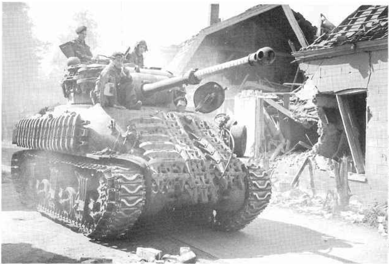
A Sherman Firefly, modified with extra armour, of the 5th Canadian Armoured Division, moves through the town of Putten, Holland, 18 April 1945.
