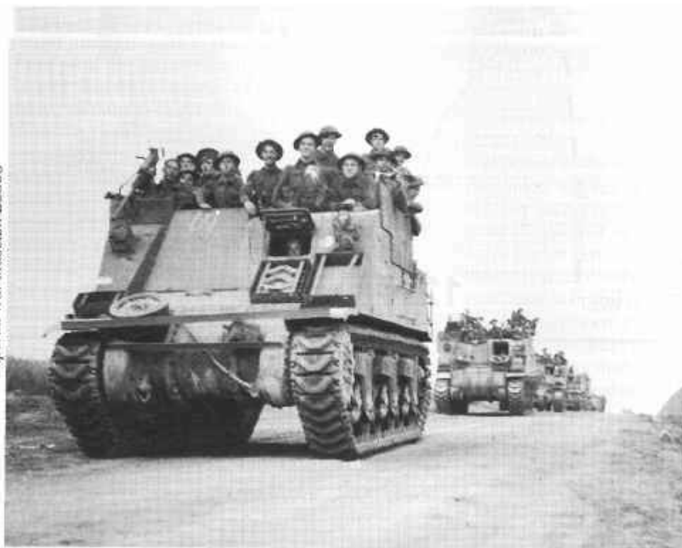
A column of "unfrocked Priests"-M7 SPs converted to armoured personnel carriers - with troops from the 51st Highland Division, 7 August 1944
