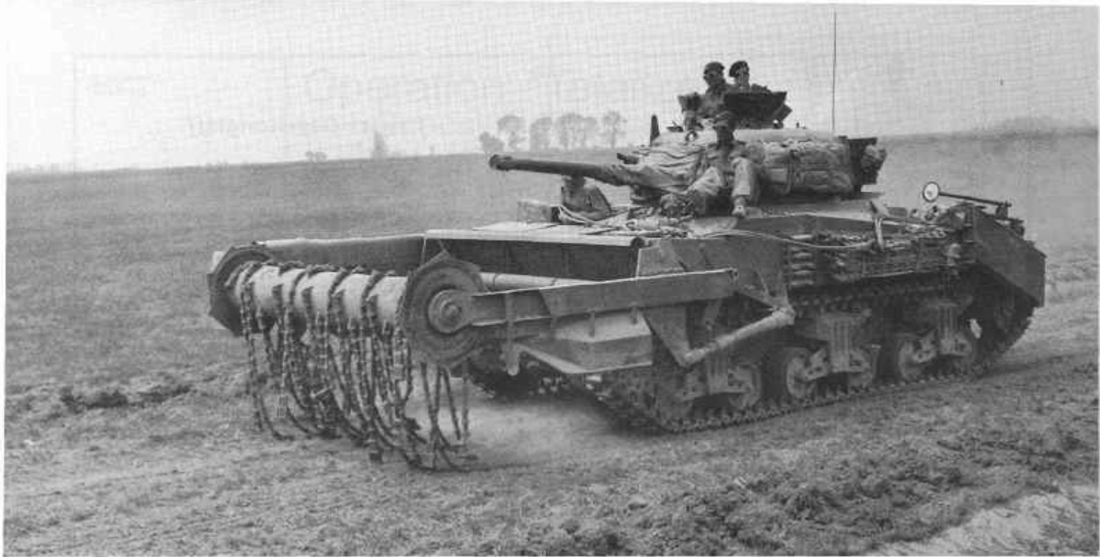
A Sherman Flail tank, crucial in Simonds' mind, to deal with the "monster minefield" which lay in the path of the Canadian advance.
