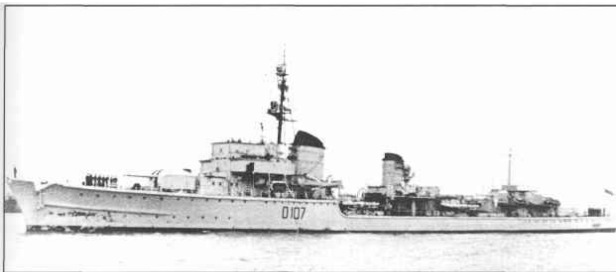
Although this post-war shot shows a sister ship qfZ-32 in British markings, it nonetheless provides a good view of a Type 36A Narvik. Note the twin 5.9-inch turret forward and three single mounts astern; her two quadruple banks of torpedo tubes are fore and aft of the second funnel.
