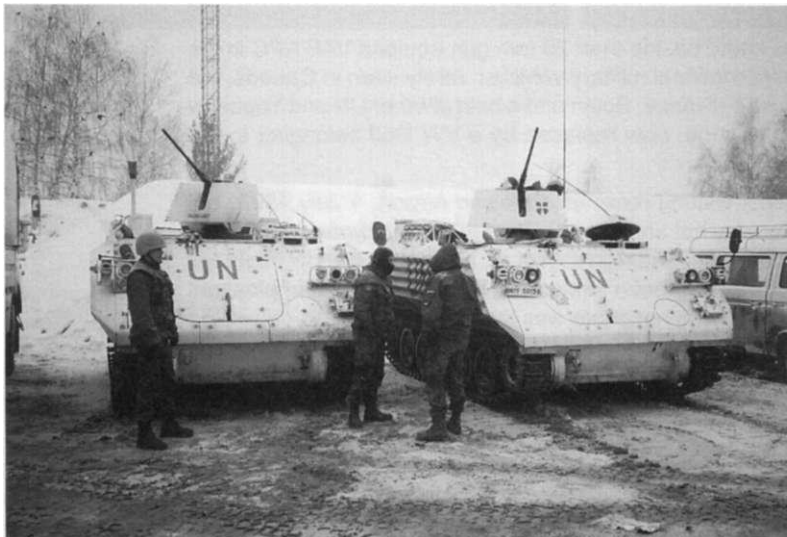
Then (below left): A Danish M113A1 APC in the parking lot of the Sarajevo Airport. This was the standard UN "taxi" for personnel in the city. The armoured shields on the crew commander's hatch and for the pintail mounted .50 cal. M2 Heavy Machine Gun are commonly referred to as Armoured Cavalry (ACAV) Shields as these were first used by the US Army Armoured Cavalry units in Vietnam in the 1960s. Now (below right): The taxis now park a little further down, to the left of the photograph, in order to pick up fares from the newly renovated and repaired terminal. Note that the International Red Cross Volkswagen Golf carries both the red cross and red crescent symbols in recognition of the Christian and Muslim populations in Bosnia.
