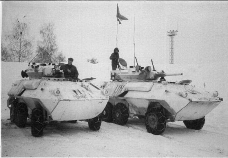
Then (above left): A pair of Canadian Cougar Armoured Vehicle General Purpose (AVGP) at the Sarajevo Airport. Chains are a must on wheeled vehicles, especially those that travel outside of populated regions as the infrastructure to clear and repair the antiquated 1950s-style Bosnian road network had disintegrated during the conflict. Now (above right): The tower with the lights are the base of comparison and the true size of the Airport parking lot is evident in this photograph. Note also the Dobrinja suburb which stretches off into the background as well as the snow on top of Mount Trebevic.
