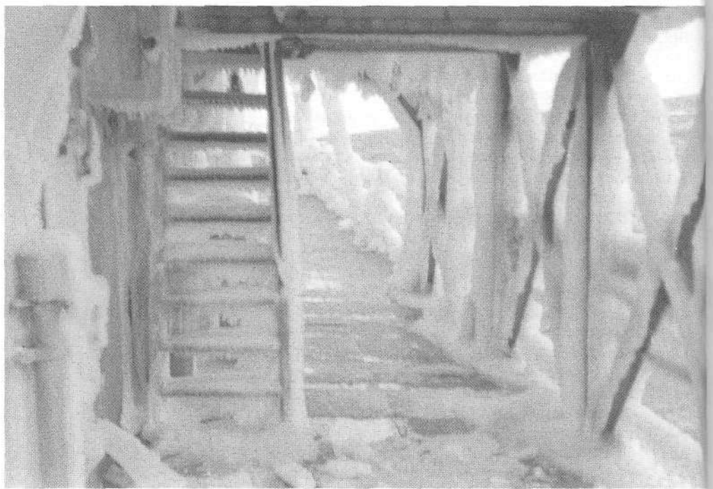
Photo 10: View down the starboard side during winter conditions. Uneven icing conditions frequently made ship handling, especially steering and staying on course, extremely difficult. Making one's way along a narrow passageway such as this one was a dangerous but routine occupational hazard for the crew. The slanted horizon line shows that the ship was rolling at the moment the photo was snapped.
